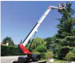
The U-1570 Evo uses Multitel's aluminium boom coupled with AlmaCrawler's bi-levelling tracked undercarriage
