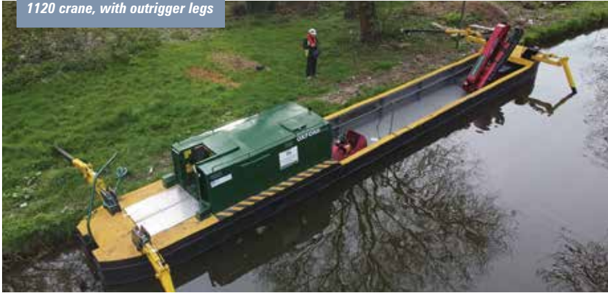
The Rothen Group's new crane boat, Oxford, carries a HMF 1120 crane, with outrigger legs
