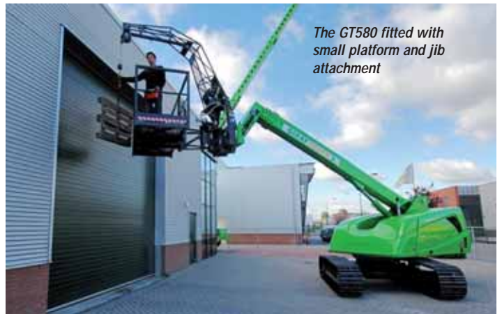
The unit can lift 750kg at 15.5 metres on a slope of 7.5 degrees
