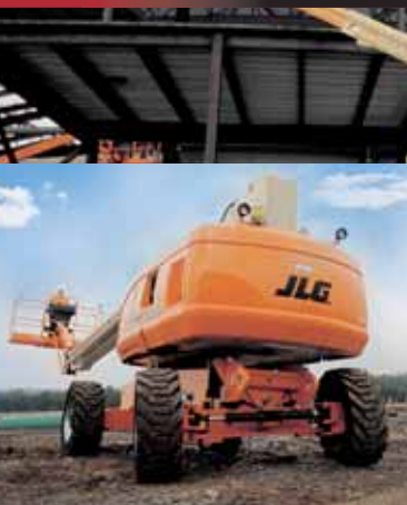
The JLG 860SJ was the first 80/86ft telescopic boom to dispense with extending axles
