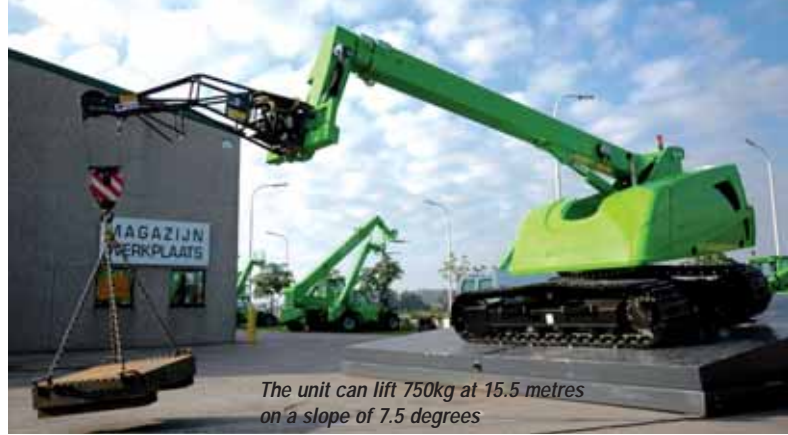
The GT580 fitted with small platform and jib attachment
