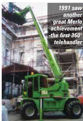
Merlo's SM25P was the first low boom, side engine fixed frame telehandler.
