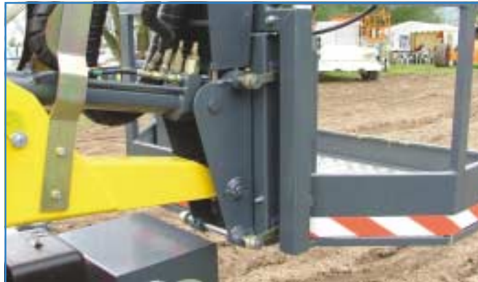
Leguan has developed this overload system for its range of skid steer boom lifts that uses an open parallelogram connection between the basket and boom. It is combined with a heavy duty spring and two micro switches, all of which are well protected from the elements.
