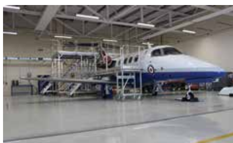
A Planet Platforms purpose built system being used by Affinity Aerospace to work on the Embraer Phenom 100
