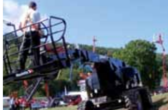
The Haulotte HA20PX scored well, although it did lift a wheel on the course.
