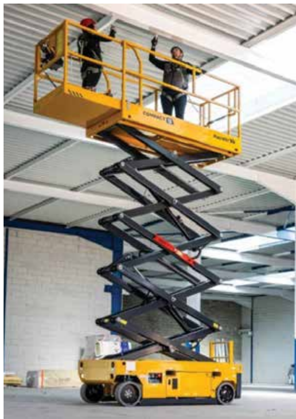
The Haulotte Compact 12 with AC direct rear wheel drive
