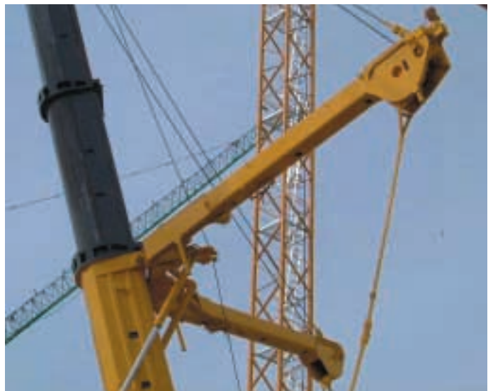
Grove's 'Mega-Wing Lift' boom support system
