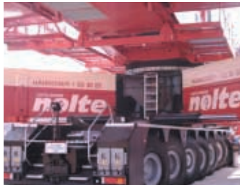
Liebherr's new 750 t capacity LTM 1750 lattice-boom mobile crane truly had to be seen to be believed. Displayed in the colours of Germany-based crane rental firm, Hans Joachim Nolte Auto-Krane, the massive unit combines a newly-developed eight-axle carrier with the upper of Liebherr's LR 1750 crawler crane.
