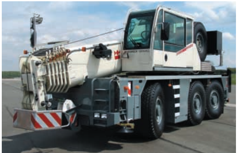
Terex-Demag's new AC 55 with the classic city 'drop-nose' boom concept first seen on Kobelco's two-axle, 7 t capacity RK70 introduced in 1989.
