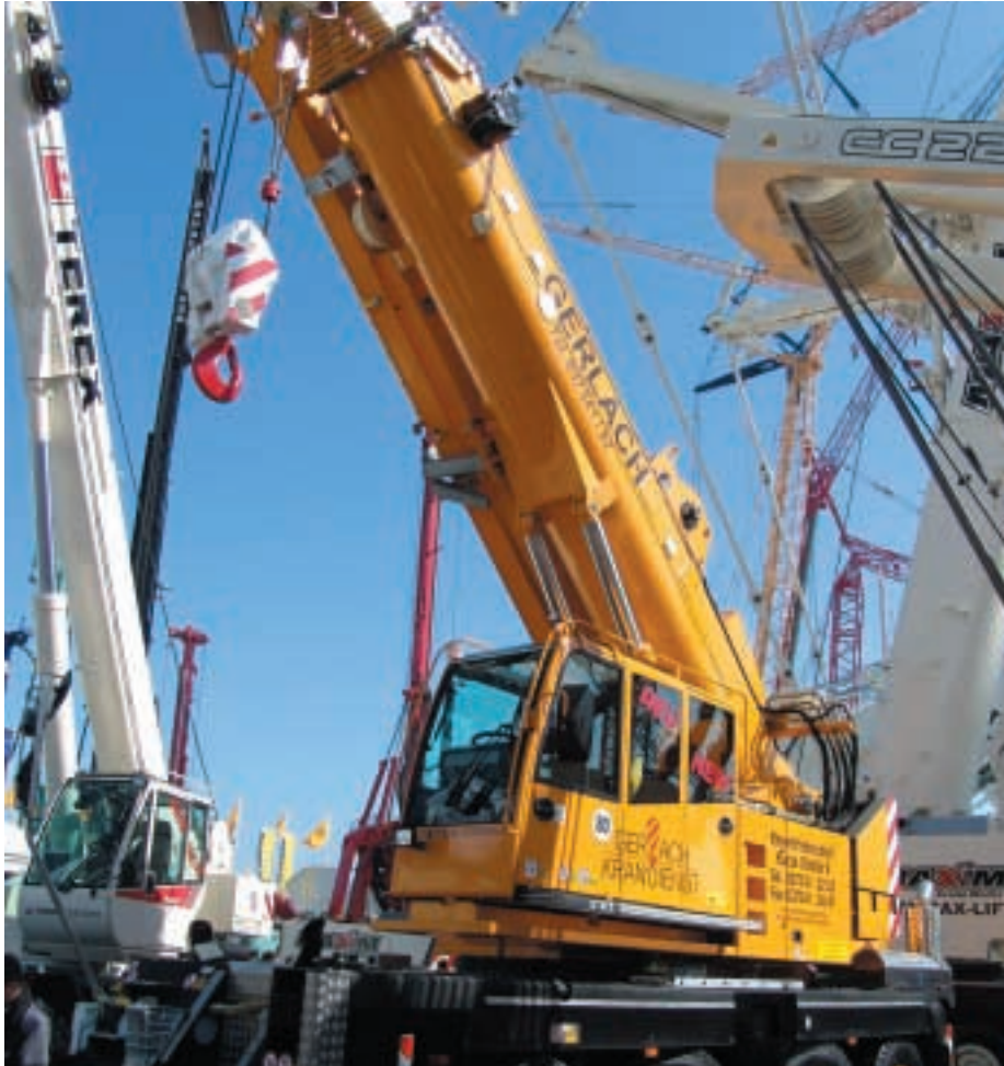
Terex-Demag's AC 70 launched at bauma 2004 replaces the 60 t capacity AC 60 and offers increased lifting capacity by way of an additionally mountable counterweight plate, also used on the new AC 55.
