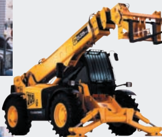
JCB boosted its Loadall telehandler range with the release of its 13.8 m lift height, 3.5 t payload 535-140 (pictured), while it also introduced the 540-170, with an improved lift capacity over its 532-120 predecessor, and the 540-140, also with an improved lift performance over its 537-135 predecessor.
