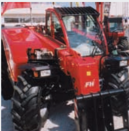
Another flagship machine, the Faresin-Haulotte partnership produced the latest 'Toplift' FH 17-40 with a 17 m lift height and a 4 t lift capacity.
