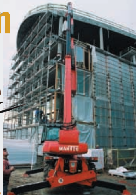
Manitou introduced its 24 m lift height, compact chassis MRT 2540 with a maximum reach of 18.5 m, now the largest machine in the company's heavy-duty telehandler line.
