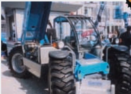
New from Genie was its Terex Italia-built 7 m working height Gladiator II GTH-3007 telehandler, which has replaced the first Gladiator model.
