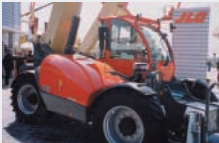
JLG used the bauma show to debut its largest telehandler to date, the 17 m, 4 t capacity 4017 based on its 4000 series, but with an extra fourth boom section.
