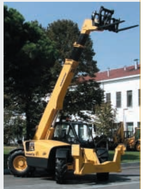
From Komatsu came two models from its new six-strong "super-low profile" series, the 12.7 m, 3.5 t capacity WH613 (pictured) and the 14.1 m, 4 t capacity WH714.
