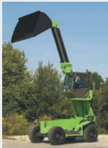
German producer, Sennebogen, displayed its unique 5 t capacity, 7 m lift height 305 Multihandler, which features a cab that can be raised to around 4 m up the boom of the machine.
