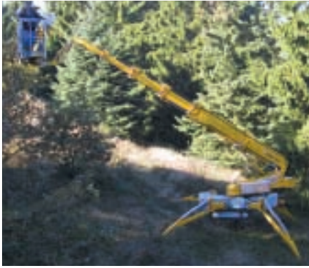
Omme produces a full range of telescopic trailer lifts and pioneered the 'drive from the basket' self-propelled function. Pictured is the 22 m working height 2200 RBD.
