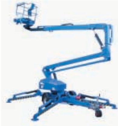
Seen at bauma 2004 was UpRight International's new 17.2 m working height UI50T.
