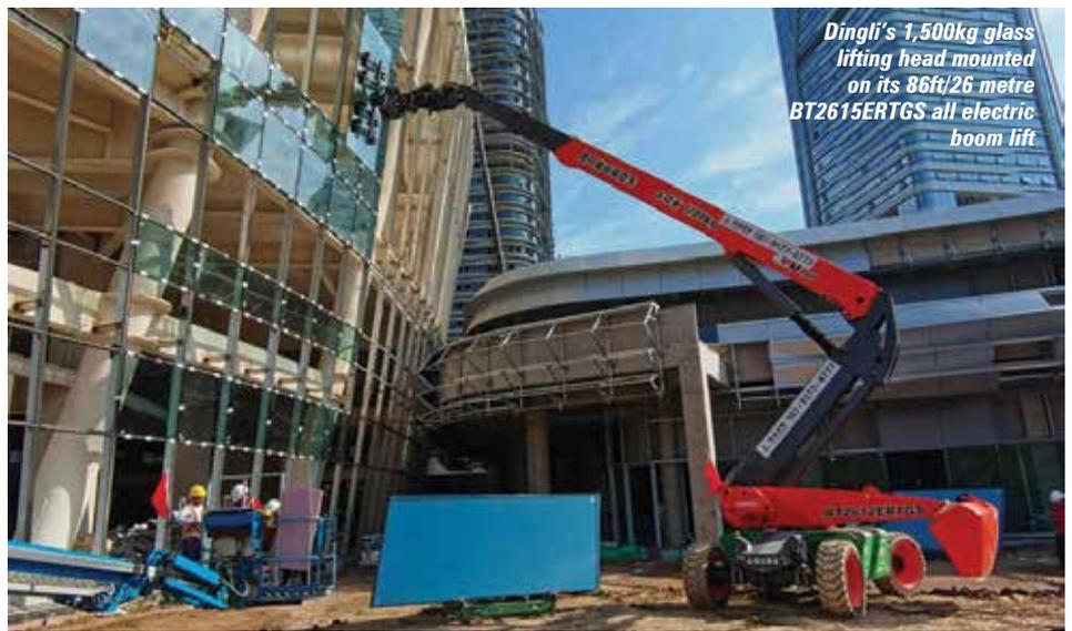
Dingli's 1,500kg glass lifting head mounted on its 86ft/26 metre BT2615ERTGS all electric boom lift
