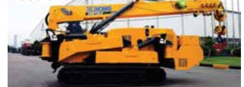
XCMG's new spider crane - the 5.5 tonne ZQS125-5
