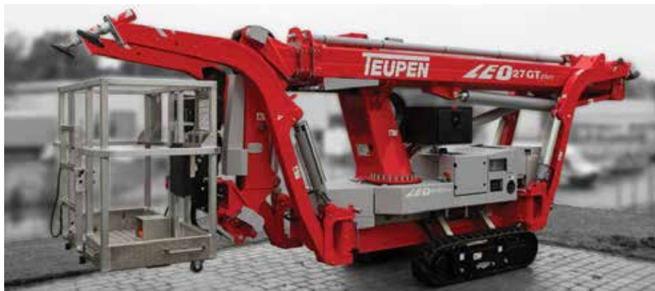
The new lift has a wide selection of set up positions and a high degree of levelling
