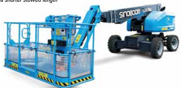
Sinoboom's TB14J Plus in Europe or TB460J Plus in North America features a three rather than two section boom resulting in a shorter stowed length
