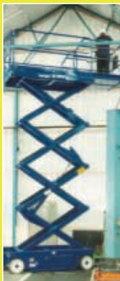
UPRIGHT X26N (SELECTION OF) – ELECTRIC SCISSOR LIFT 10M WHT 2000
