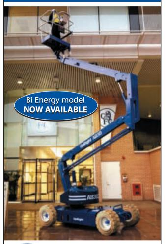
UpRight AB38/AB38 Lite-micro-booms with maxi-performance. Packed with class-leading compact features, the UpRight AB38 micro-boom has a 13.45m working height, and 6.10m of
