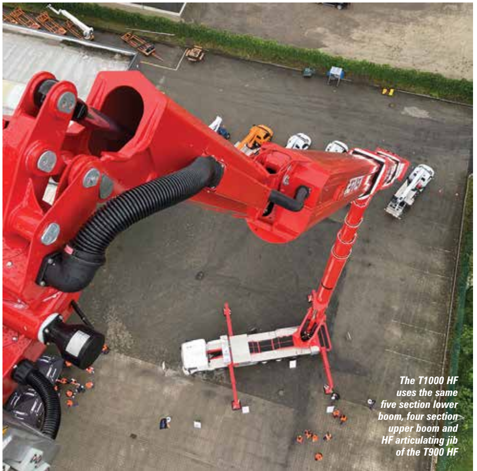
The T1000 HF has a 3.82 metre by 970mm extended platform - seen here at the launch event
