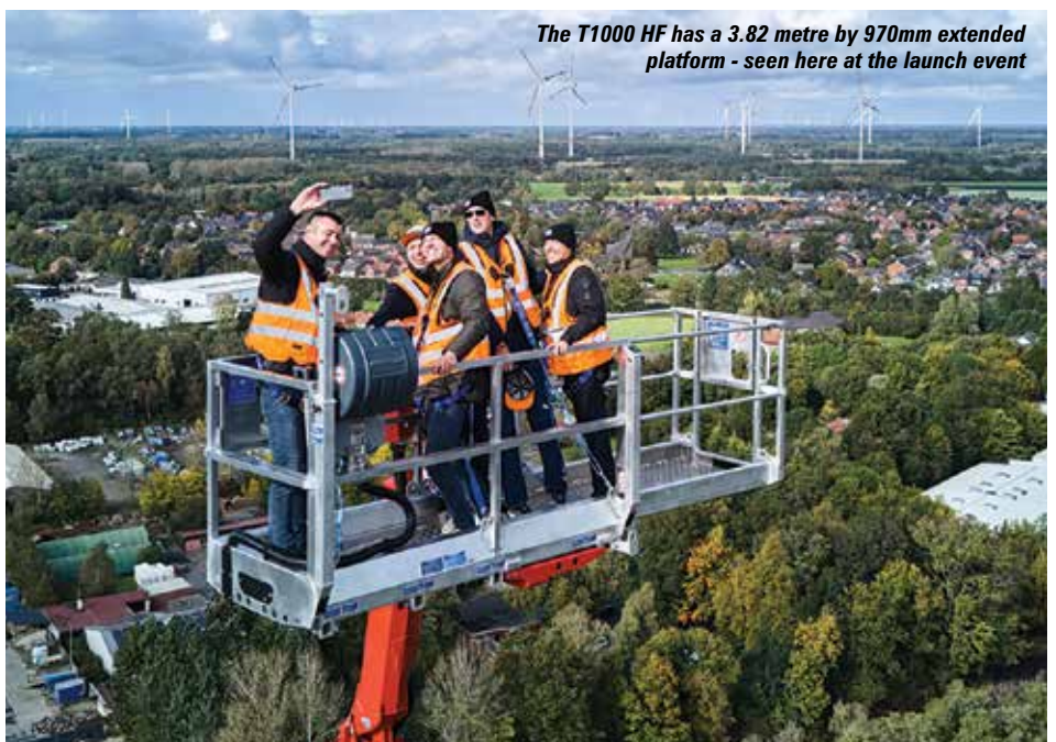
The T1000 HF uses the same five section lower boom, four section upper boom and HF articulating jib of the T900 HF
