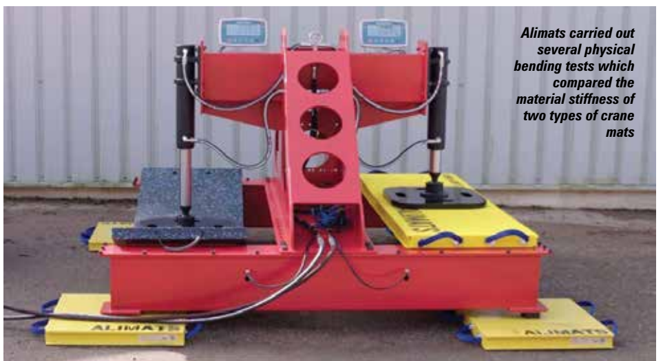
A material that is strong in compression is not necessarily stiff. Hardwood is stiffer than softwood, nylon and polyethylene
