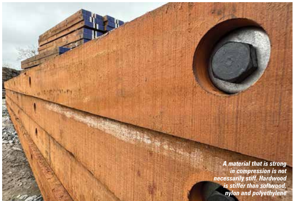
Alimats carried out several physical bending tests which compared the material stiffness of two types of crane mats
