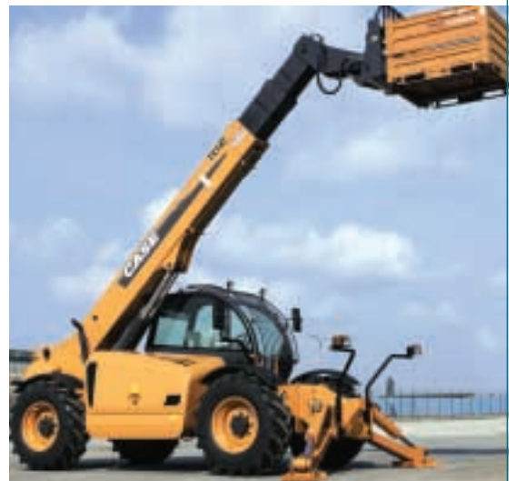
This 14 metre lift height TX140 from Case is the first model to be unveiled from its all-new 3 strong telehandler range. The full line, including the 12.45 metre TX130 and the 16.6 metre TX170 will be available later in the year.
