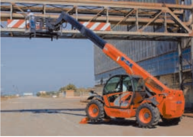
Fiat Kobelco's 14 metre T14 sits half way in its new Evolution range, which also comprises 13 and 17 metre lift height models.
