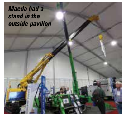
Of note on the Movex stand was the tracked carrier based 500kg telescopic crane...
