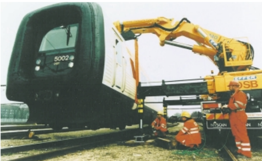
The Effer 140 Rail Road Crane will soon be replaced by the 2100 version, capable of lifting 31 tonnes at a 4 metre radius and 13.5 tonnes at a 12 metre radius. The new rail / road worthy model has been designed to meet the extremely stringent specification requirements of the UK rail network.
