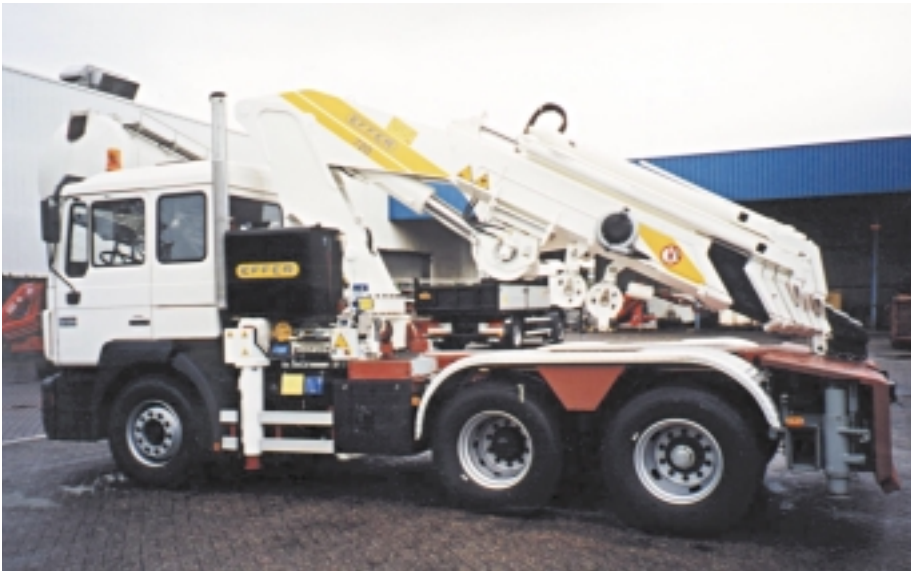
Effer's 70 tonne/metre 720 knuckle boom crane models are available with capacities up to 220 tonne / metres. When mounted on a 3 or 4 axle truck, its 'city class' characteristics makes it a seriously viable alternative to truck cranes in the same class.
