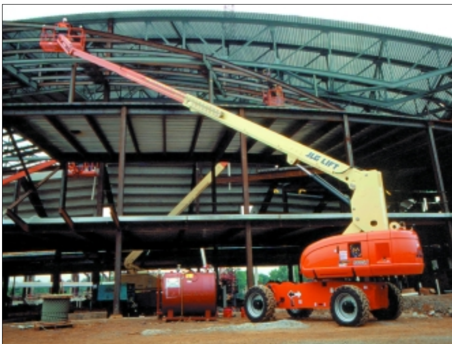
A special boom design from JLG allowed for a narrow machine width and low gross vehicle weight on its 800 Series platforms
