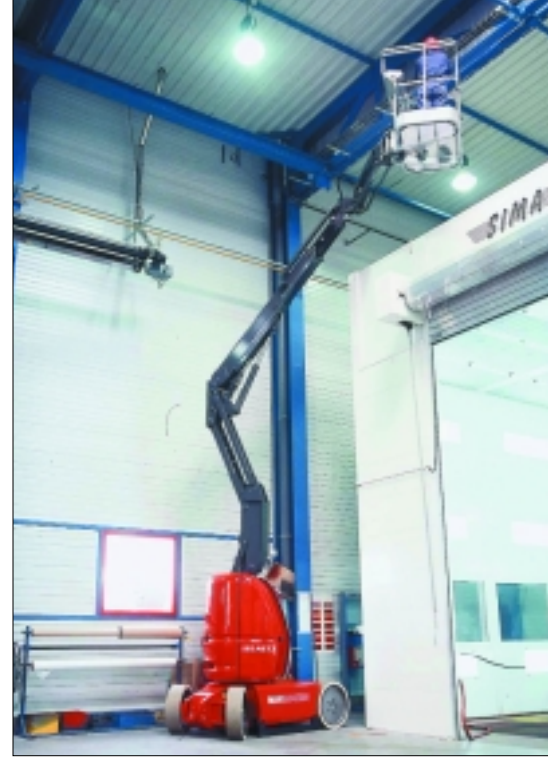
The soon to be launched 120 AEJ articulated boom from Manitou is just 1.2 metres wide and provides a working height of a 12.2 metres
