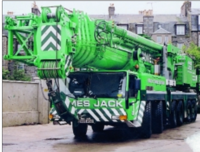
James Jack Lifting's 300 tonne capacity LTM 1300/1a
