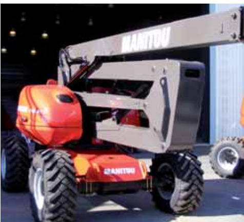
The new Manitou 200 ATJ boom has a new over-centre riser design.
