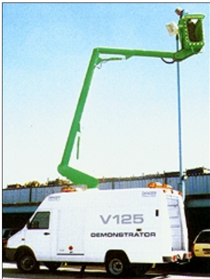
The Niftylift V125 has plenty of storage space and a useable payload of 500 kilograms
