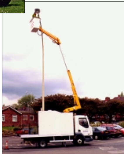
Dudley Metropolitan Council's new Versalift ETN38NF platforms, with 110 degree flyboom
