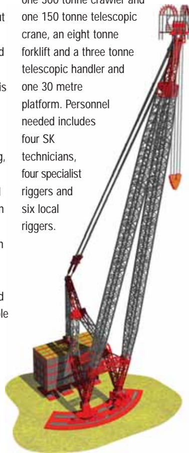
The AL.SK90 'lifting machine' can be equipped with a standard winching system for weights up to 600 tonnes and a strand jack system for loads up to 4,300 tonnes.
