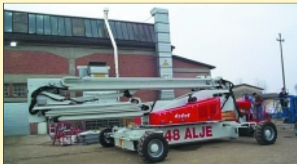
The newly launched Basket Sel 48 ALJE-D, with a 48 metre working height and 23 metre outreach.
