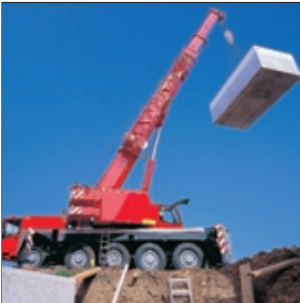
The Demag AC100, with the shortest chassis at 11 metres
