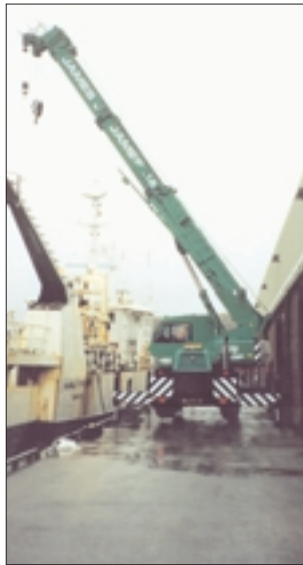
Kato CR250 25 tonne city crane on a Scottish harbour
