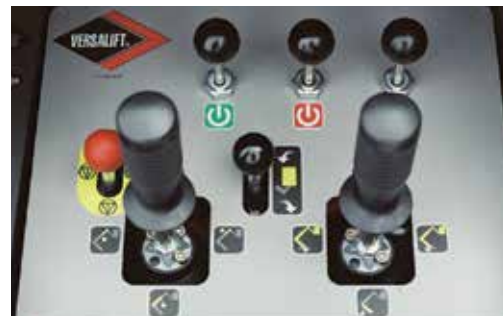
The new fully hydraulic twin joystick control system.
