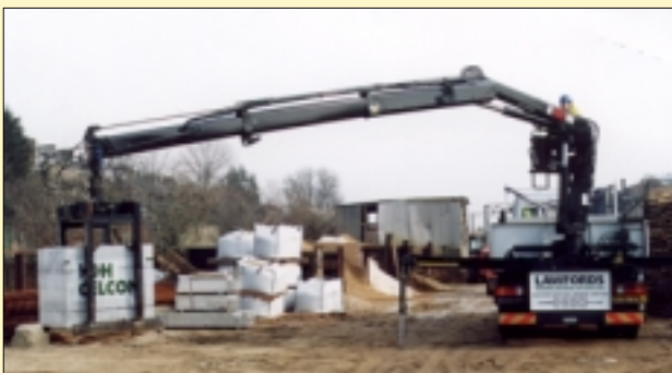
London based Lawfords has taken delivery of three more Hiab lorry-mounted cranes. The cranes are two 102 knuckleboom on two new 26 tonne, six-wheel Mercedes vehicles and an O85-2. All three were supplied with the optional top seat control system as Lawfords believes this allows safer and more efficient handling.
