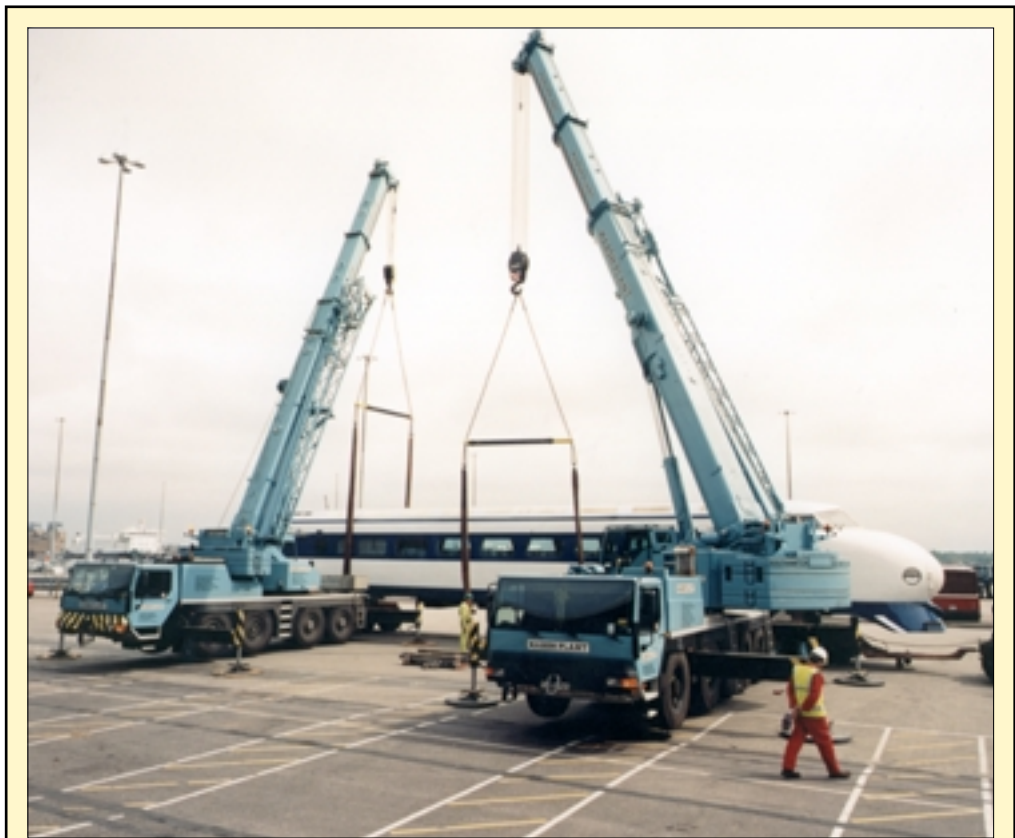
This "Shinkansen" bullet train recently arrived at Southampton docks where Marsh Plant Hire used its new 100 tonne Liebherr LTM 1100/2 and 80 tonne LTM 1080/1 to unload the precious cargo. Bullet trains can travel at more than 200 kilometres per hour – this one, a gift from the Japanese people, travelled rather more slowly by road to the National Railway Museum in York.
